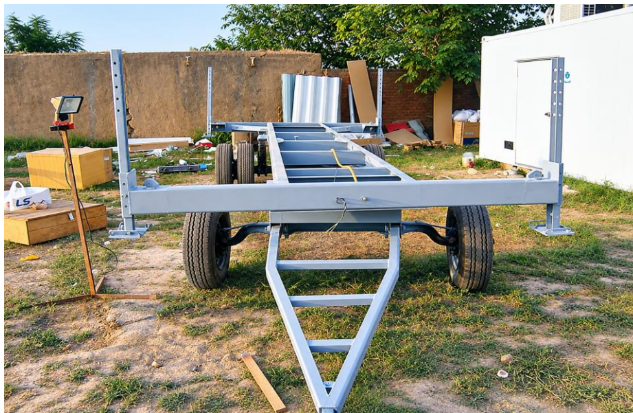
Prefabricated facilities portfolio | Transportable-unit chassis and fabricated frame
